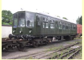
Guard's van of this vehicle progressing too, with the correct type of doors in the process of being fitted to the driver's side. The driver's side of the roof has been wire brushed ready for painting.
